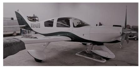
The aircraft is a kit developed by Express Aircraft Company and features a cantilever low-wing, four seat cabin, fixed tricycle landing gear with wheel pants, and a single engine in tractor configuration. It is full VFR and Kelley runs a Lycoming IO 540 engine which offers a cruising speed of 210 mph. The aircraft features a fiberglass body and wing. It was finished in March of 2005, just months prior to his move north.
