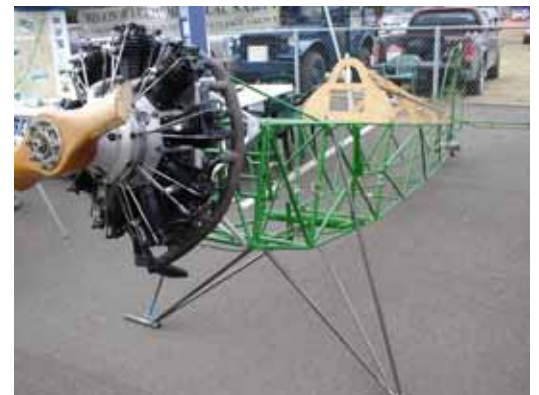
Salmson 40hp Engine mounted on the Rupert Special after approximately 60 years apart!
