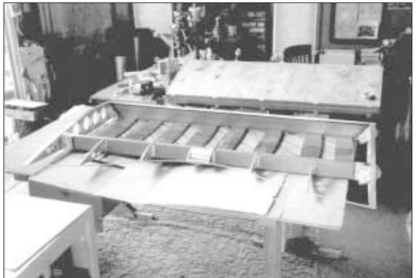
*Photograph being sent by regular mail: Our new center section wing, and the donated tin plate fuel tank. The aluminum parts in the new fuel tank bay are baffles for the new tank.*
